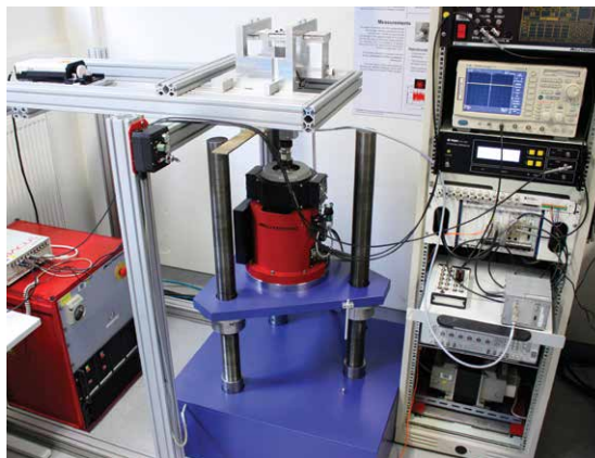
Figure 12: Device for dynamic torque calibration at PTB.
