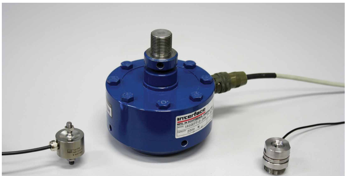
Figure 1: Three force transducers investigated in the scope of the project EMRP IND09 (from left to right): HBM U9B / 1 kN, Interface 1610/2.2 kN, Kistler 9175B (-8 kN...30 kN).
